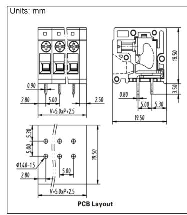
Housing: PA66, UL94V-0 Pin: Copper Alloy, Tin Plated
